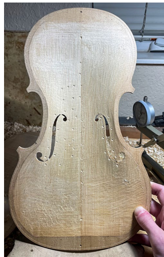
Image 3: planed to .2-.3mm above final thickness.
