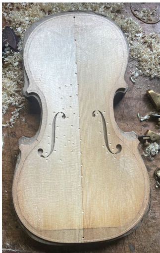
Image 2: planed to .5mm above final thickness.
