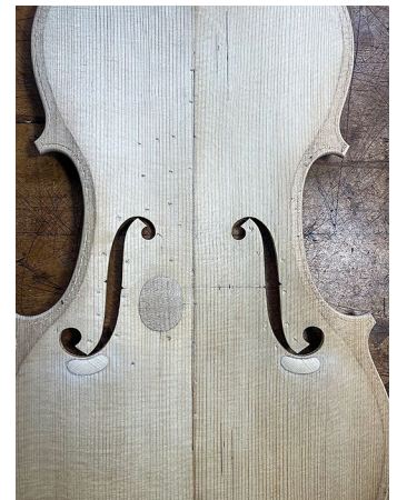
Image 5: The sound post veneer and cleats at the f holes are glued in and shaped for reinforcement. You can see what is left of the holes.
